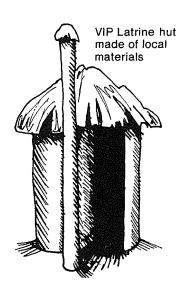
ZIMVIP (Zimbabwe Ventilated Improved Pit Latrine). Its main innovation is a super structure with a spiral cross section.
