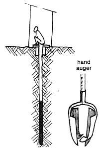
Borehole latrines. These can be quickly constructed with a hand augur. They are especially useful where a quick sanitation solution is essential (eg. refugee camps) and where people are likely to move around regularly. However, the small diameter of the hole means that it is likely to foul, block and fill quickly.
