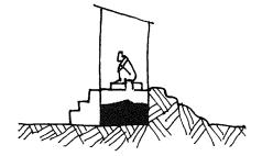
**Mound or step latrine.** This type is suitable for areas where you cannot dig into the ground, eg. where the water table is high or there is hard rock near the surface. However, the user is close to the excreta.
