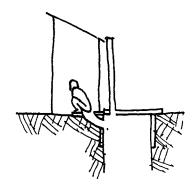
Offset latrine. The waterseal and seat can be on firm ground. The pit can be in softer, easier-to-dig ground, and can be protected to prevent collapse. The slab can be small, as it does not have to act as a lid for the pit, useful where cement and other reinforcement are difficult to get.
